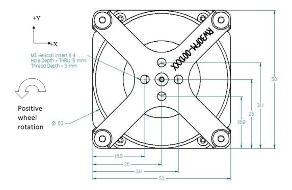
The X and Y axes are defined as shown in the figure. The Z-axis (illustrated in the following figures) completes the right-handed set. The rotation arrow shows the direction of wheel rotation that is considered positive speed. Rotation in the opposite direction is considered negative wheel speed.
