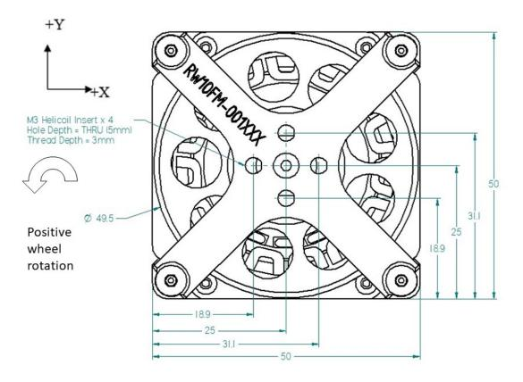
The X and Y axes are defined as shown in the figure. The Z-axis (illustrated in the following figures) completes the right-handed set. The rotation arrow shows the direction of wheel rotation that is considered positive speed. Rotation in the opposite direction is considered negative wheel speed.
